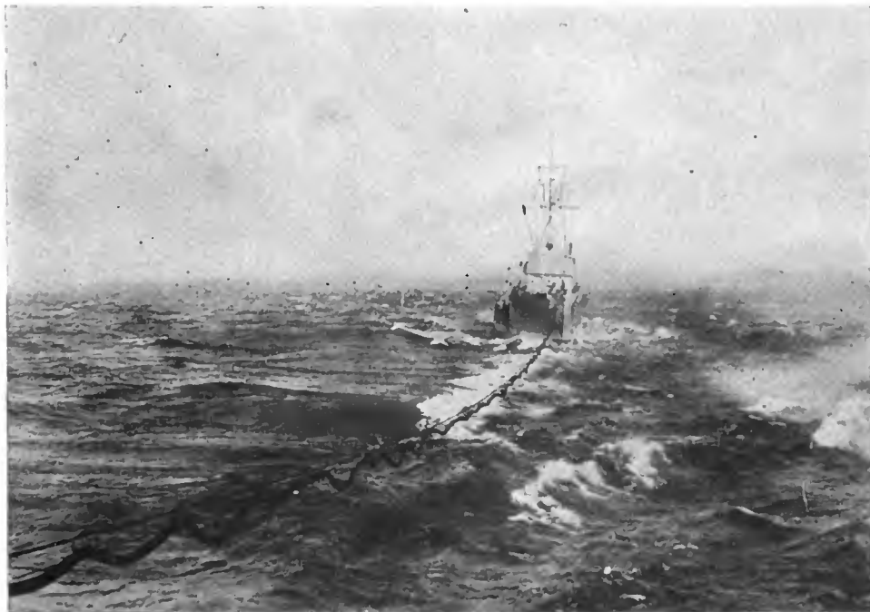
The new method of supplying fuel to destroyers at sea is revealed in this view of an oil hose attached to a tanker
