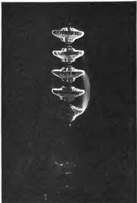
High tension insulator tested under oil up to 300,000 volts
