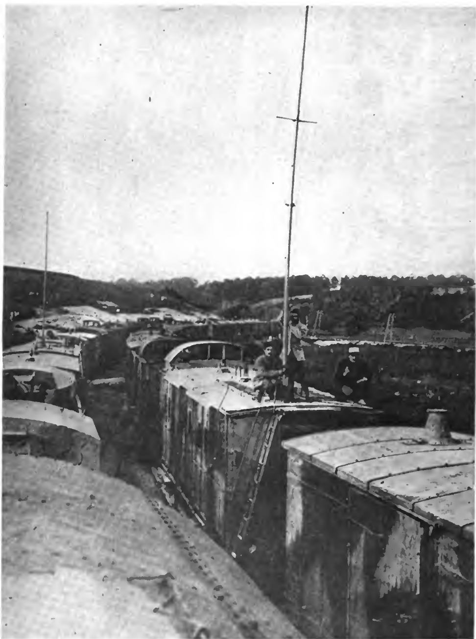
The lessons learned in peace times through the equipment of passenger railroad trains with a wireless dispatching system, are given practical application to war problems. The photo shows French soldiers at work erecting a wireless outfit on the top of a camouflaged train in the Marne district
