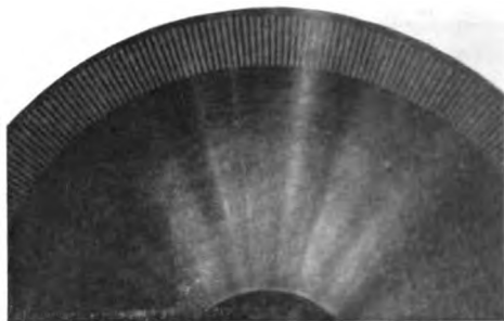
Figure 105—Portion of rotor of Alexanderson 100,000 cycle alternator, showing slots in disc
