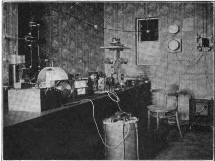
Figure 33—Ruhmer's radiophone transmitter
