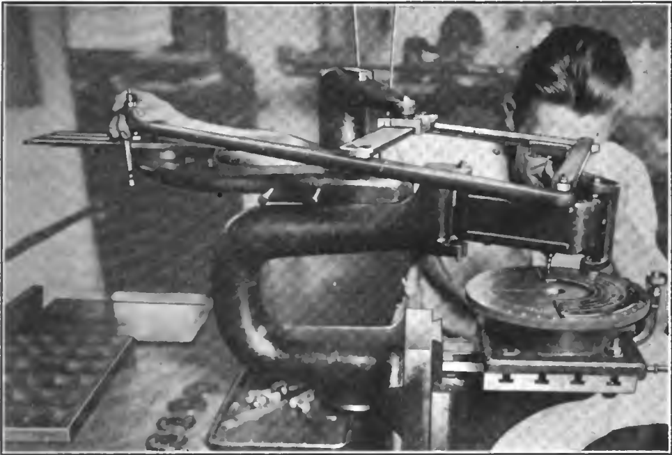
Making the fine recording scales and dials of the wireless instruments on a machine which operates on the pantograph principle. Various forms of engraving tools are used, according to the fineness or coarseness of the lines
