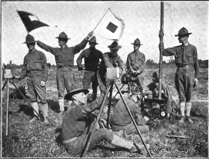
Illustrating two visual and one electrical means of signaling; heliograph and wigwag at left, wireless on right
