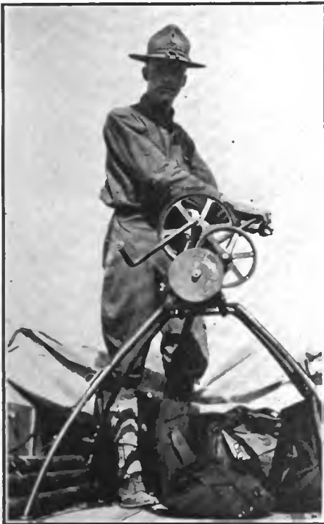
The hand generator which supplies current to the back wireless set of the Signal Corps.
