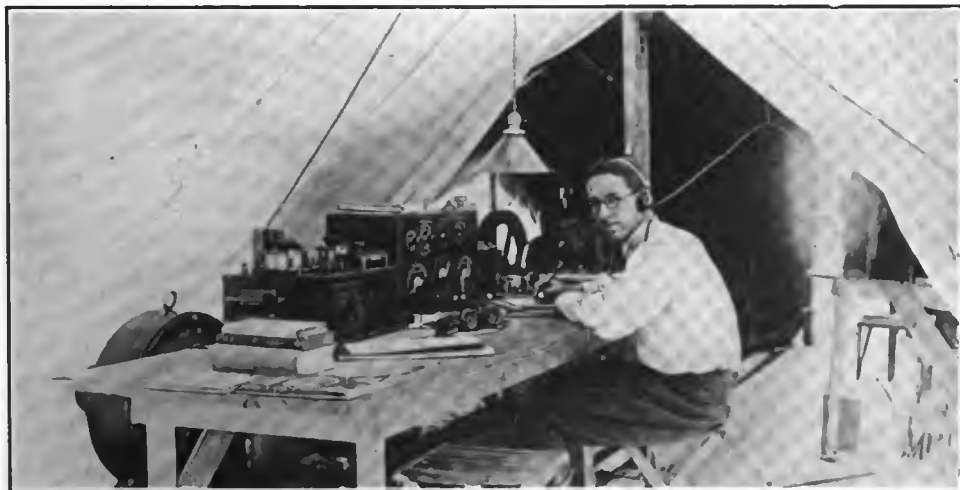
Interior of the wireless station, Lieut. Hotchkiss at key of the 2 k.w. Marconi set
