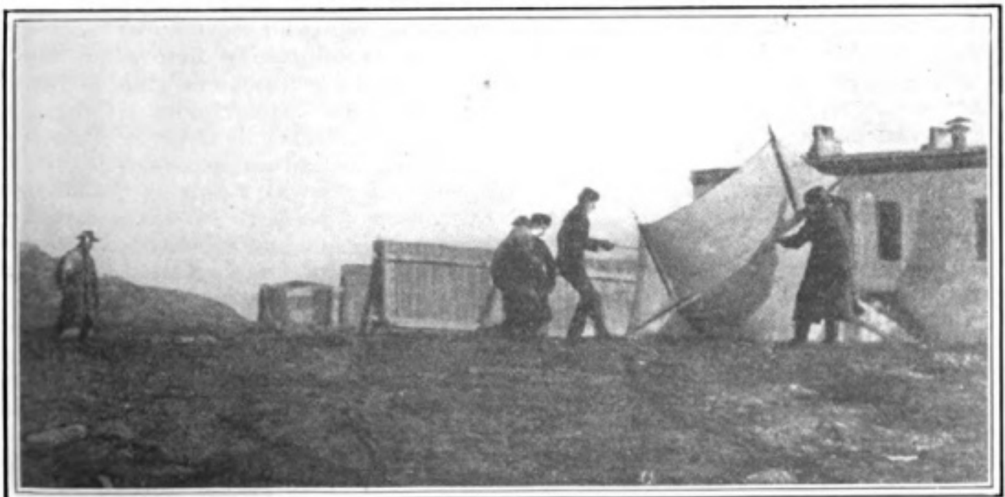
Preparing to fly the kite which supported the receiving wire. Marconi on the extreme left
