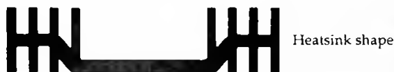
Figure 4.11 The shape of the 78xx type of stabiliser IC and a suitable heatsink.
