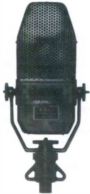
Marconi Ribbon microphone, type AXBT, used by the BBC from 1934-1959
