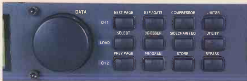
The obligatory data wheel and the 12 LED-equipped navigation buttons
