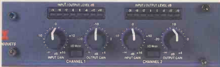
Each channel has a pair of pots for controlling input and output gain
