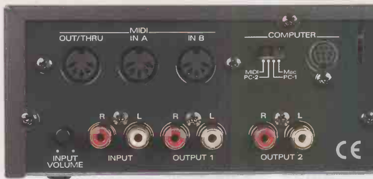
Two sets of outputs at the back, but only on phono plug
