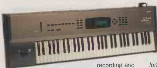
Korg a la mode: put the N364 in Sequencer mode to use multi-timbrally
