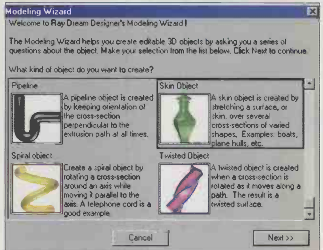
The Modelling Wizard contains a range of 3D shapes which are good starting points for your own objects.
