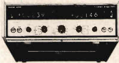
B900 Automatic Digital Bridge 1kHz 0.1%
