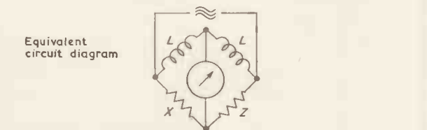
Fig. 10. Basic diagram of the reflection factor meter 3R29 for 50 to 1 000Mc/s and of the reflection factor meter 3R225 for 300 to 3 000Mc/s
