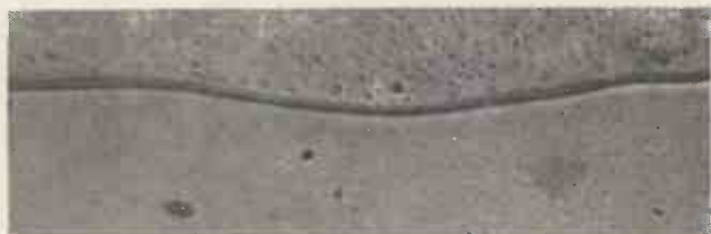
Fig. 17. Electropolished precision-drawn brass waveguide surface from 1\text{in} \times \frac{1}{2}\text{in} guide Section from long side parallel to waveguide axis Magnification: 940 Brass in lower part of photograph
