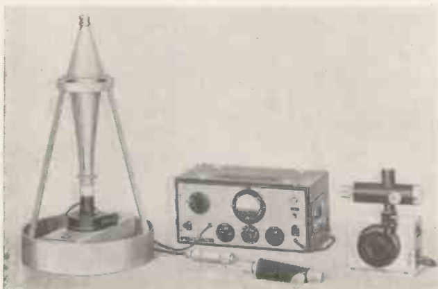
Fig. 7. Thermal wattmeter with terminal resistor (left) and wattmeter multiplier, with blower for cooling (right)
