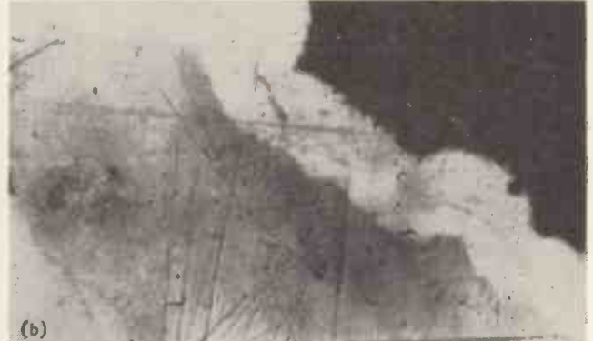
Figs. 22(a) and (b). Electroformed copper waveguide surfaces from 1in x 1/2in guide. Composite stainless steel mandrel. Copper cyanide bath Sections perpendicular to waveguide axis Magnification: 940 Copper in lower part of photographs
