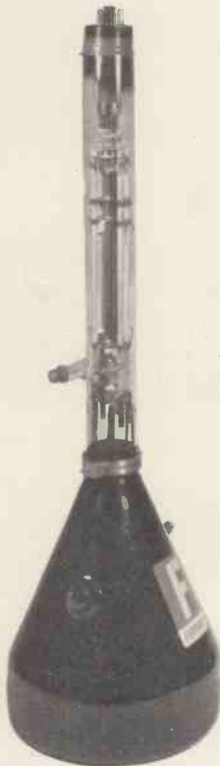
Fig. 1. Prototype of the high current transient oscillograph cathode-ray tube with an experimental low sensitivity signal deflector coil
