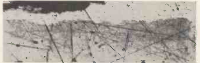
Fig. 7. Precision drawn copper waveguide surface from 1\text{in} \times \frac{1}{2}\text{in} guide. Section from long side parallel to waveguide axis. Magnification: 940. Copper in lower part of photograph.
