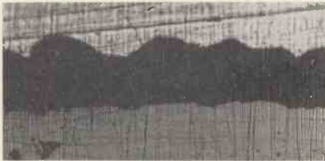
Fig. 11. Acid copper electroplated brass waveguide surface from 1\text{in} \times \frac{1}{2}\text{in} guide. Section perpendicular to waveguide axis. Magnification: 950. Brass in lower part of photograph and acid copper plating in the dark band.
