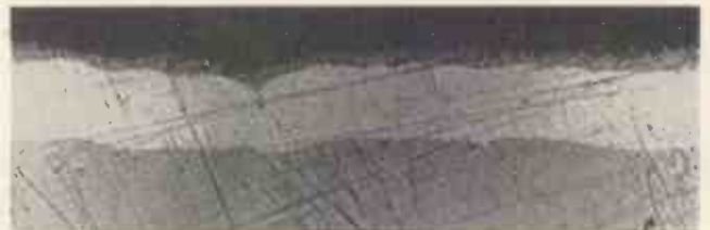
Fig. 12. Cyanide silver electroplated waveguide surface from \frac{1}{2}\text{in} \times \frac{1}{2}\text{in} guide. Section perpendicular to waveguide axis. Magnification: 980. Cyanide silver plating in the light band and brass waveguide in the lower part of the photograph.
