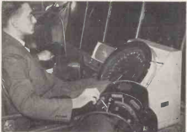
Interior of crane operator's cabin, with television screen displaying image of ingot.
