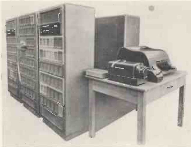
Fig. 3. The digital computer with its teleprinter and tape reading unit
