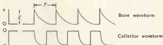
Fig. 4. The base and collector waveforms
