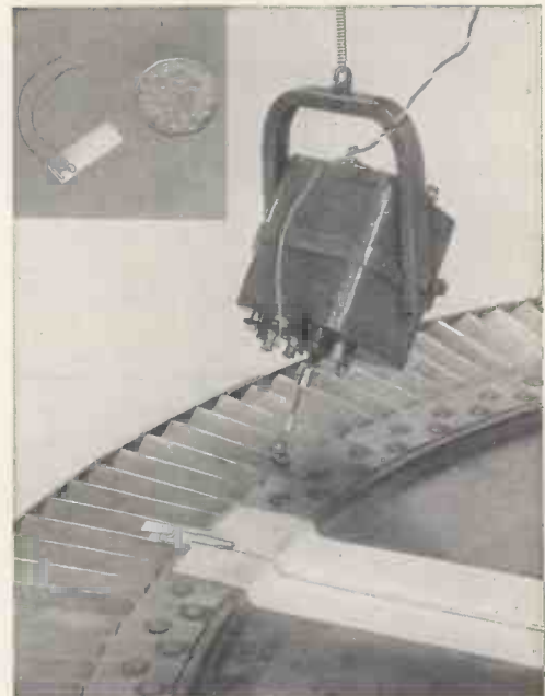
A comparison between two methods of vibration measurement on a turbine blade. In the foreground is a new G.E.C. Barium Titanate Vibration Strain Gauge and behind it the much bulkier equipment for the electro-dynamic measurement of vibration.
