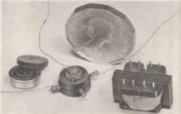
Fig. 12. Toroidal-shell transformer, and conventional type of equal ampere-turns performance
