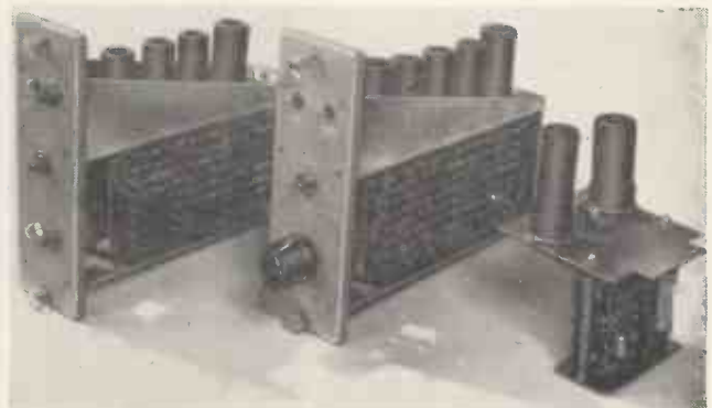
Fig. 4. Gate units and reset pulse stage
