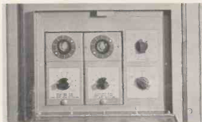
Fig. 10. The front cover of the tray opened to show the controls. The machine is set at "Seam" 8c/s "Cool" and 8c/s "Heat".
