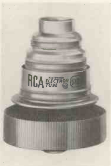
Fig. 5. RCA type 6181 v.h.f. power tetrode. Output power 1 200W at 900Mc/s.
