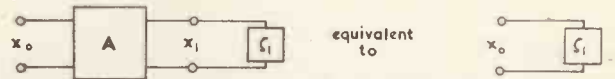
Fig. 10. Illustrating the fact that the input impedance of an infinite chain is unaltered by removal of one quadripole
