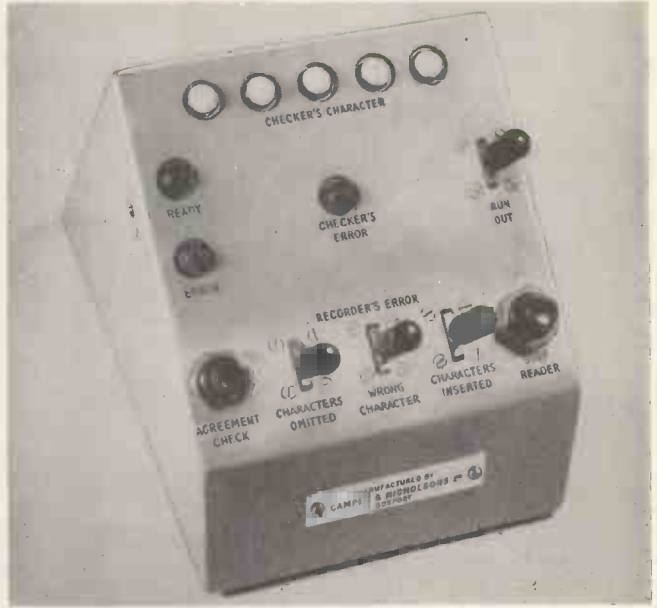
Fig. 19. The control panel showing the keys, lamps and buttons required for correcting errors
