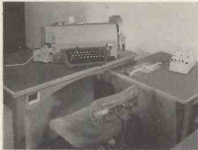
Fig. 28. General view of the tape checking device showing the teleprinter, tape reader and control panel
