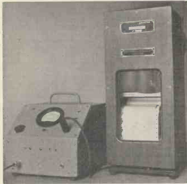
Fig. 5. The Boyd Research Trust Cardi tachometer with the Evershed and Vignoles pen-recorder
