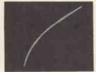
Fig. 17. 7475, 20c/s, 5mA, D.C. (Large current swing)
