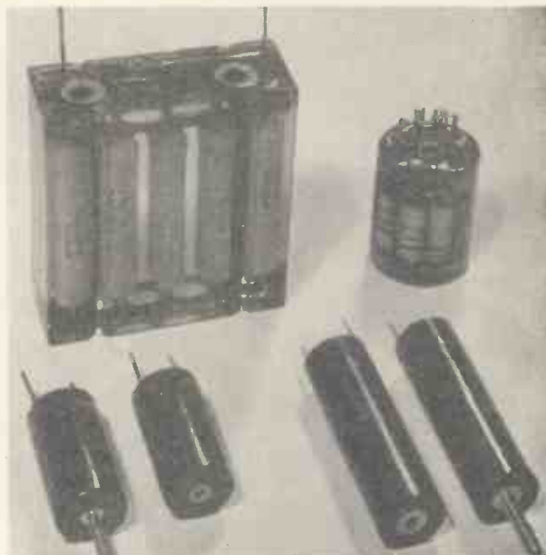
Fig. 1. Resistors potted in Araldite D (By courtesy of Evershed & Vignoles Ltd.)
