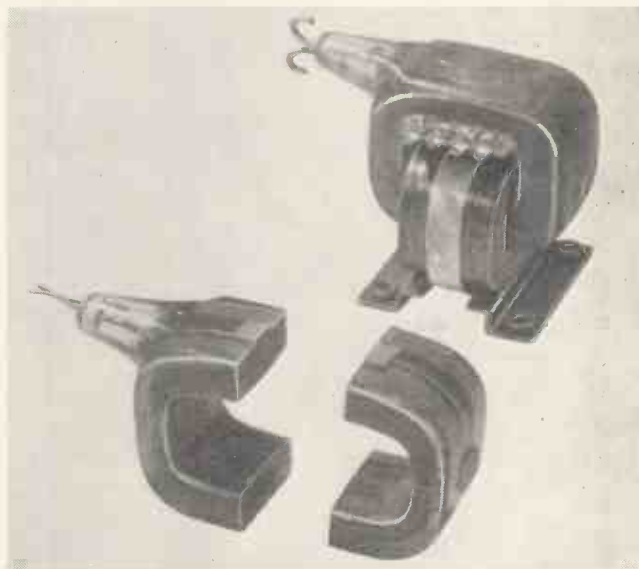
Fig. 4. Pulse transformer embedded in Araldite casting resin B (By courtesy of Aircraft Transformer Co., U.S.A.)
