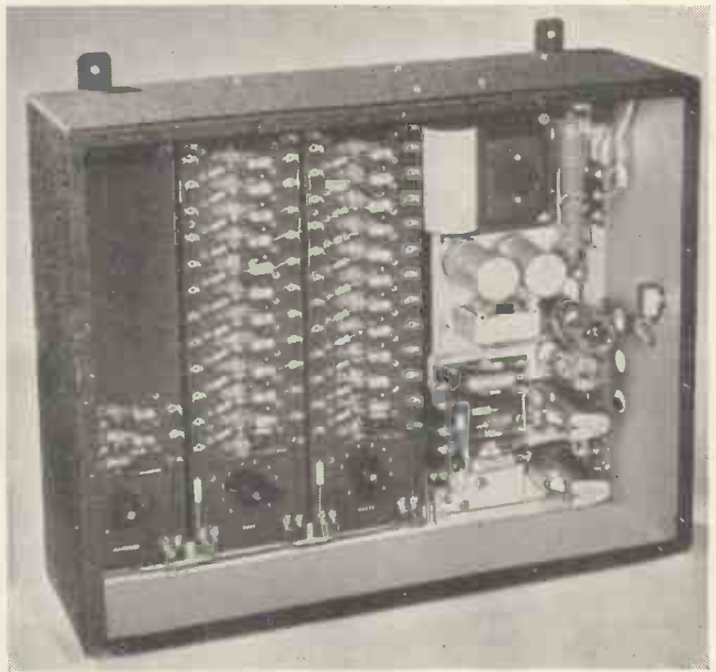
Fig. 2 (below). View of counter with front cover removed
