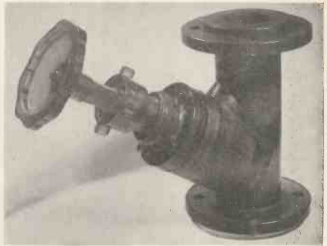
Fig. 8. Valve for chemical plant cast in Araldite casting resin B. The bore of the valve is 4 in.
