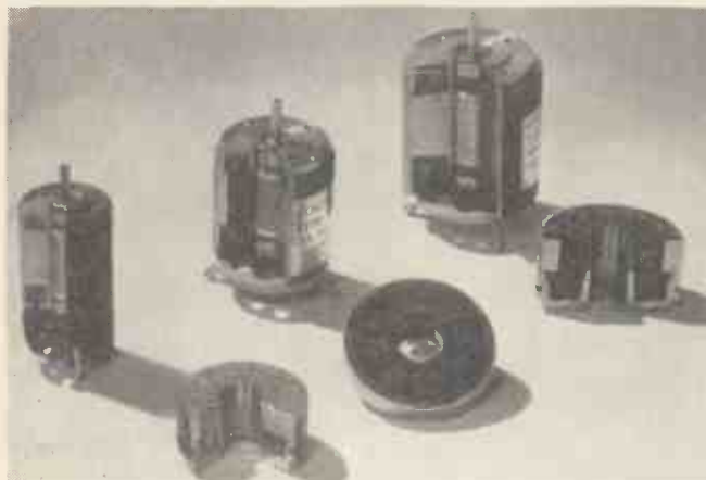
Fig. 5. Servo motors. Laminations bonded with Araldite 15, potted in Araldite casting resin B (By courtesy of Kearfott, Co., U.S.A.)
