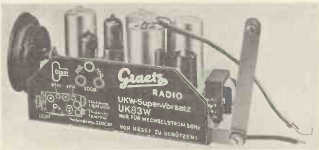
A simple v.h.f. adaptor made by Graetz Radio for use with broadcast receivers. It consists of a 9-stage 3-valve circuit with 2 germanium diodes and a metal rectifier power supply. The price is 109DM (about £9).
