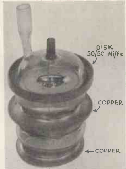
Fig. 6. Envelope for the ACT25 U.H.F. disk seal triode
