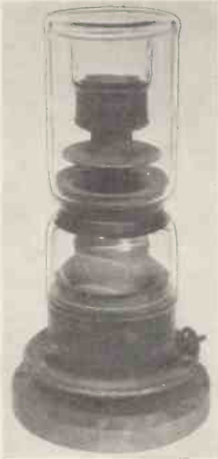
Fig. 5. Double insulator used in mercury arc rectifiers
