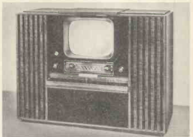
A luxury type radio and television receiver made by Nora. This instrument contains a 40-valve television receiver with a 21in tube, a four-band receiver including v.h.f., tape recorder, microphone and an automatic three-speed recorder player. There are six loudspeakers. (Price 4900DM-£410).
