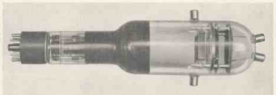
Fig. 39. (Above) the aperture of the coding tube viewed from the gun end; (below) the complete tube
