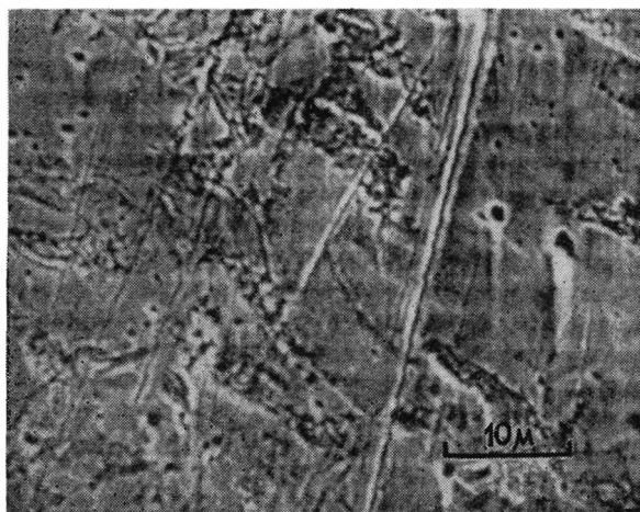
Fig. 8. Mild steel. Perpendicularly scanned, magnification \times 1500 , 15kV, 1.5 \times 10^{-10} A beam current, exposure 300 seconds
