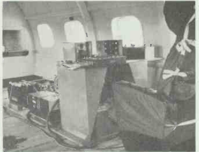
Fig. 4. Twelve-channel portable vibration recording gear installed on an Armstrong Whitworth Apollo aircraft
