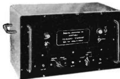
Frequency Standard—1744 —1 kc/s to 80 Mc/s—0.005% accuracy.
