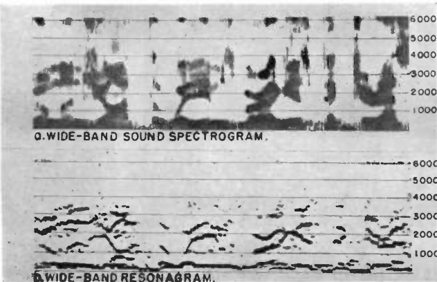
Fig. 3. Comparison of wide-band spectrogram and resonagram of some speech sample as Fig. 2
