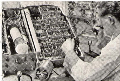
This Pye Television transmitting equipment has more than 3,000 Ersin Multicore soldered joints.
