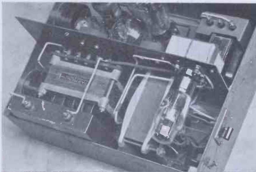
Mains equipment compartment showing location of the various compartments. Note full-wave rectifier mounted on the side wall so as to secure good heat radiation.
