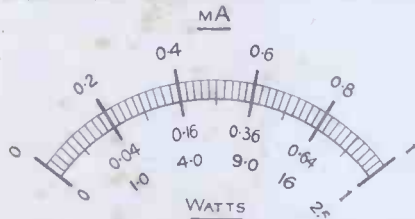
Fig. 5. 100v. and 500v. A.C. ranges in terms of watts.
