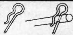
Terry's retaining pins replace the split pin. Spring grip on side holds firm. Top ring for easy removal. Sizes from 3/8" to 1 1/2".
