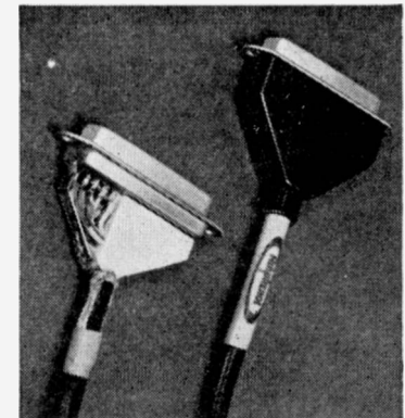
Miniature cable assembly: connector/cable junctions are potted in 'Silcoset' to protect from moisture, shock and vibration. Courtesy Amphenol-Borg (Electronics) Ltd., Northern Division.
