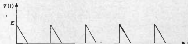
Fig. 2. Unmodulated triangularly shaped trailing edge pulses
