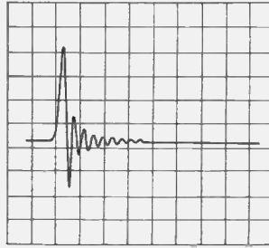
Fig. 15. Power amplifier input waveform Y = 100mV/div X = 20nsec/div
