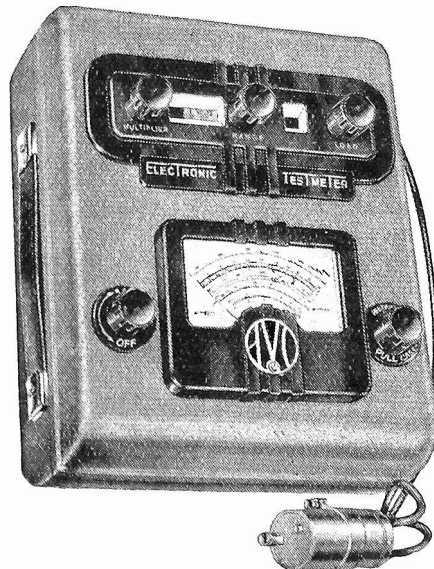
(Above) Improved universal valve tester and characteristic meter (Below) Multi-range electronic testmeter —Automatic Coil Winder and Electrical Equipment Co. Ltd.
