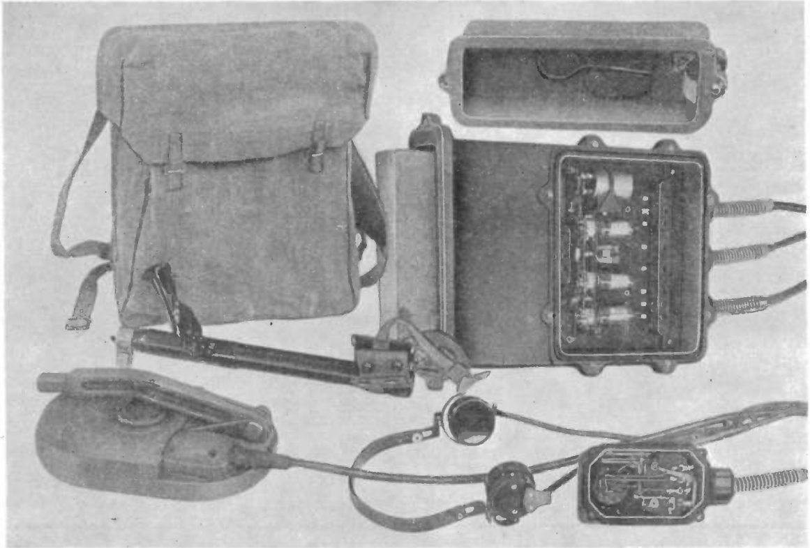
Fig. 9. Component parts of modern mine locator with cover of amplifier and control box removed.
