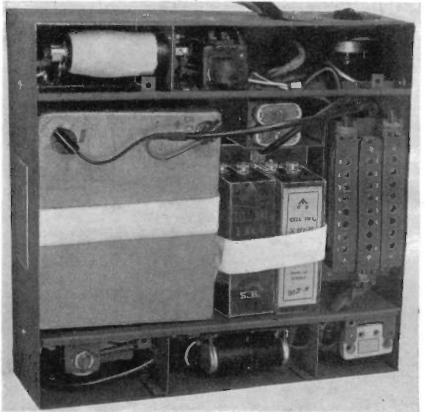
Fig. 4. Amplifier box with self-contained batteries and sub-chassis. The control is in the top right corner.
