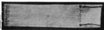
Wire resistance gauge (approximately full size). The wire is Nichrome 0.0006 in. dia., heavier leads being attached for connexion to the cable from the recording equipment. This type is wound on a paper support and the resistance is 2,000 ohms.
