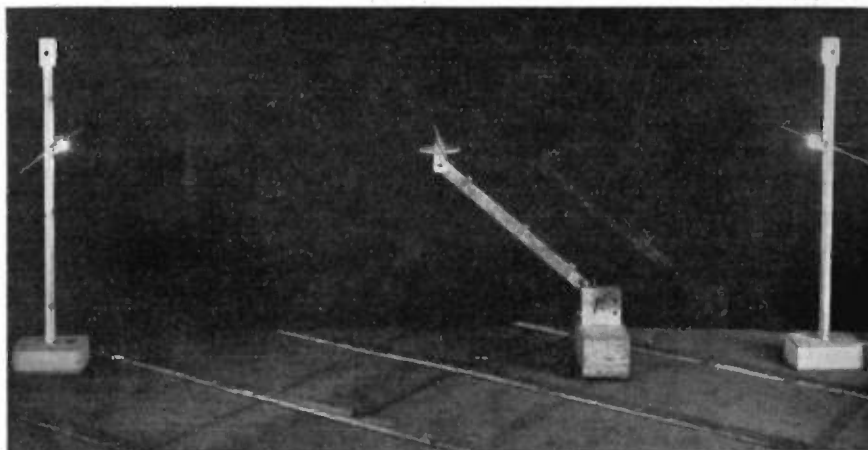
Fig. 13. Horizontal dipole with reflector. The parasitic reflector is made longer than the radiator, and placed \lambda/4 behind. The left-hand pick-up then shows the greater strength.
