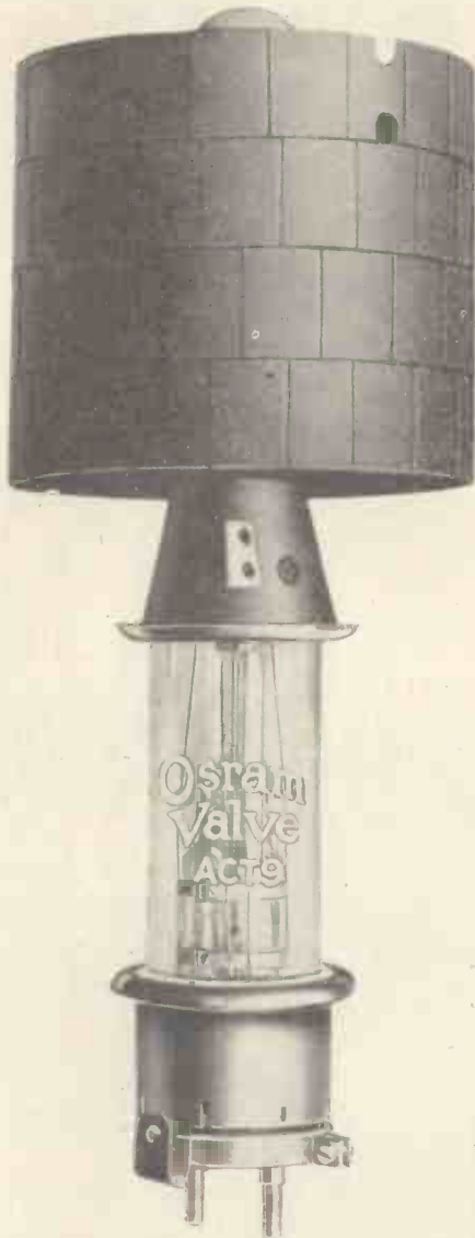
External anode fitted with radiator for natural cooling or forced air cooling, depending on the output required. Usually employed for outputs up to 4.5 kW per push-pull pair at frequencies up to 15 Mc/s.
