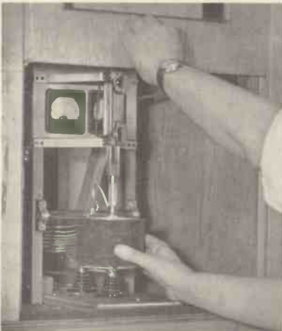
Fig. 5. Moulded preform between the electrodes in a H.F. cabinet. (By courtesy of Modern Plastics.)
