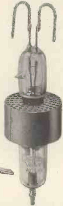
External anode air-blast-cooled triode designed for an output up to 500 W per push-pull pair at frequencies up to 100 Mc/s.
