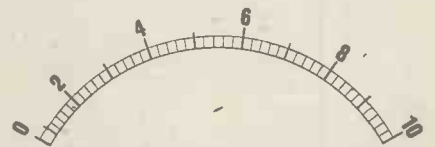
Fig. 2. Typical scale of modern moving iron instrument.
