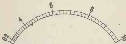
Fig. 8. Typical scale of thermal instrument. Considered as infinity in relation to the reactance of the condenser.
