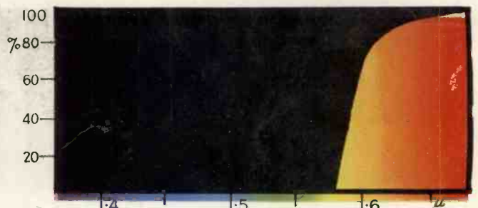
Transmission band of red filter for 3-colour photography or television.
