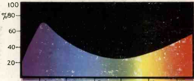
Response of Cs-Ag0 Photo-Cell for infra-red work 100% = 2 \times 10^{-3} amps/watt. Peak response to 0.85 \mu .
