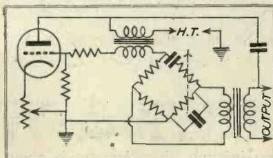
Fig. 3. Audio-frequency Oscillator using Wien Bridge.
