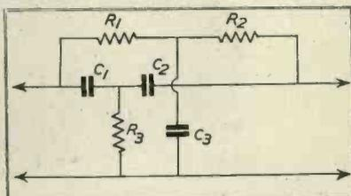
Fig. 2. Equivalent Parallel-T Network.
