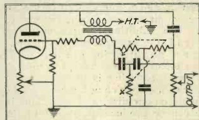
Fig. 4. Audio-frequency Oscillator using parallel-T network.
