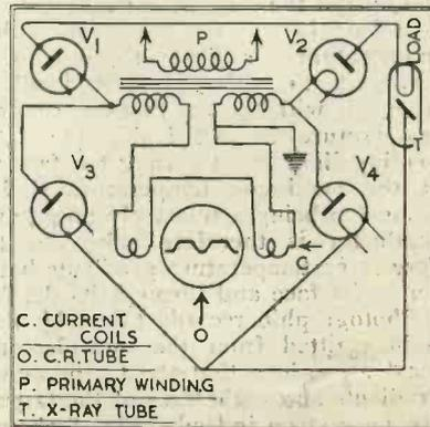
Fig. 5. Circuit for observing tube current.
