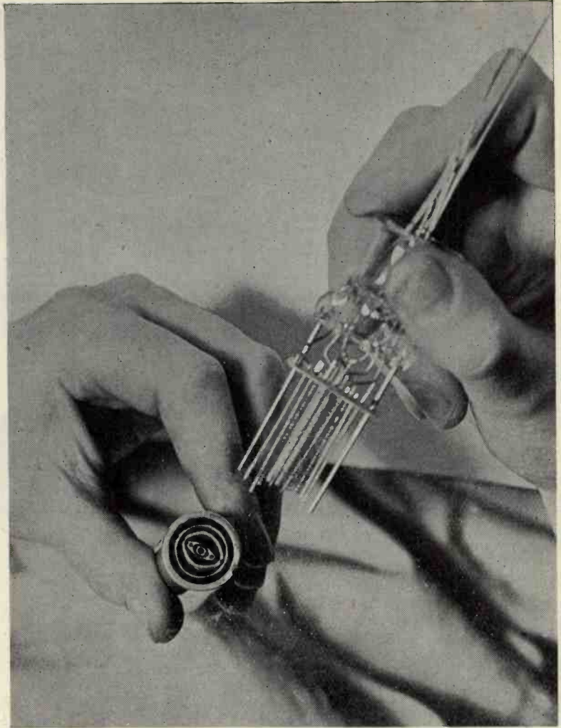
Fig. 8. Photograph of a barrel jig used in electrode assembly.
