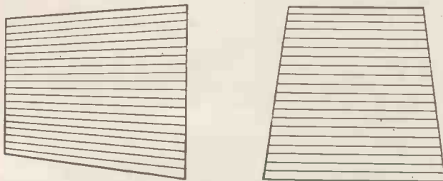
Figs. 7 and 8. Showing the effect of trapezium distortion caused by unbalanced sweep potentials. The line formation is exaggerated.
