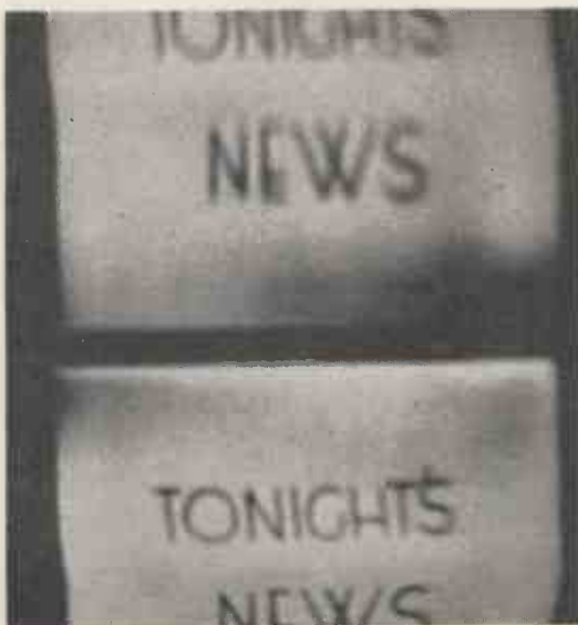
Fig. 4. Frame time base operating at one-half the correct frequency.
