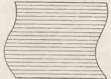
Fig. 10. A.C. ripple in horizontal (line) time base.
