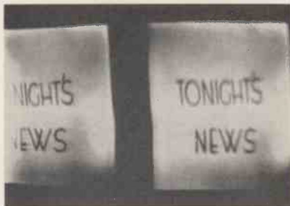
Fig. 2. Effect due to line time base operating at one-half frequency current.
