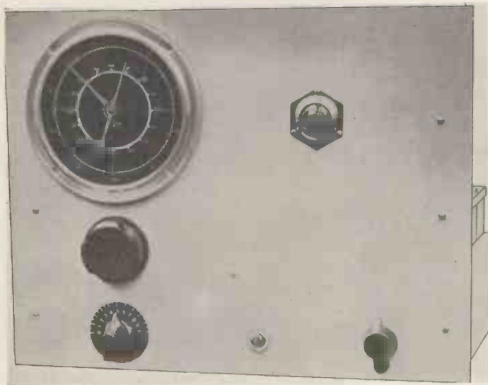
The rotary switch on the right-hand side is in the mains lead, while the toggle switch is for stand-by operation. The small condenser underneath the mains condenser is for band setting.
