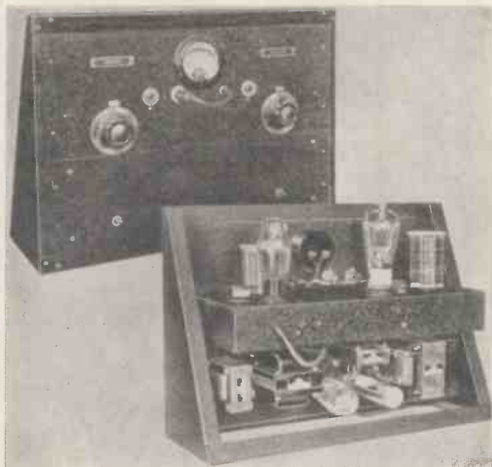
This illustration shows the construction of the completed transmitter, with the power-unit on the bottom deck.
