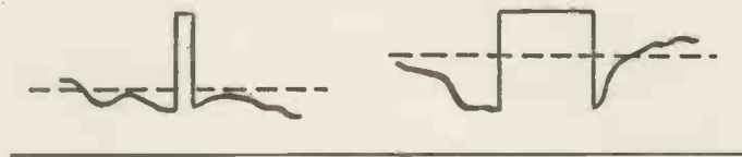
Fig. 2. In the absence of D.C. level the mean potential of the signal alters with the picture content.
