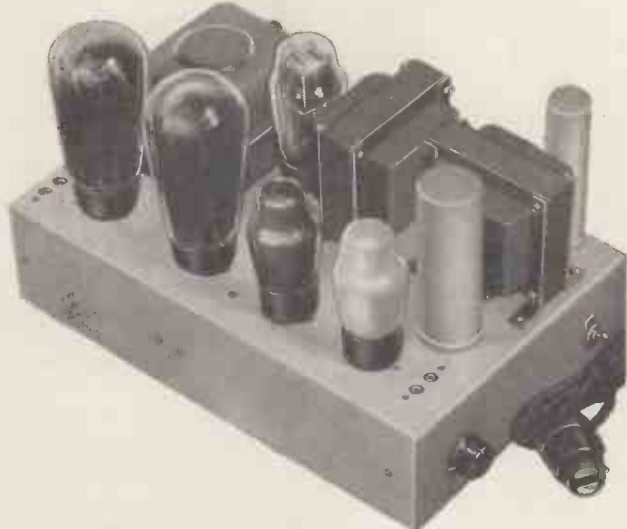
The 14-watt amplifier is completely self-contained with double smoothing. Two triodes in push-pull provide excellent quality at maximum output. As there are two drive stages, quite a small input voltage is required to fully load the output triodes.
