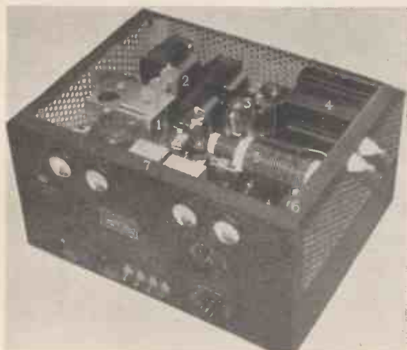
A typical Collins phone transmitter complete with power packs and modulator.
