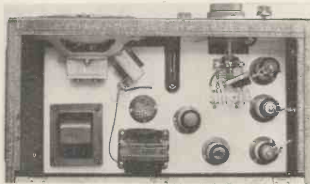
This plan view gives a good idea of the layout of the components. Particularly notice the arrangement of the mains transformer, output transformer and smoothing choke.
