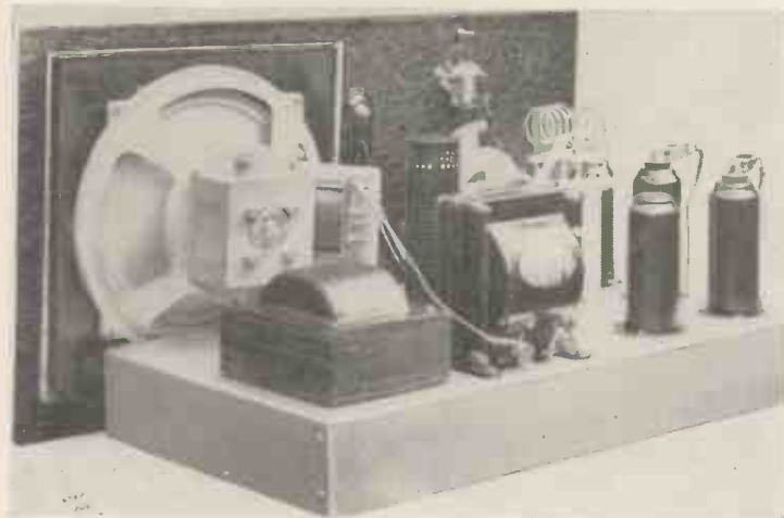
By using a special transformer, all connecting leads have been kept beneath the chassis.
