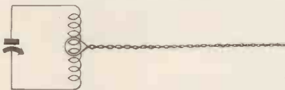
Fig. 7.—A particularly low-loss arrangement using 72-ohm cable.
