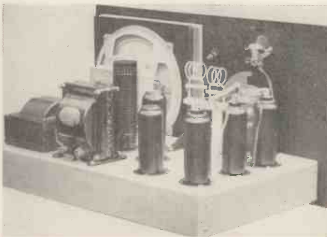
The valves shown in this illustration are from left to right, rectifier, output pentode, second detector, two I.F. amplifiers and the first detector next to the panel.
