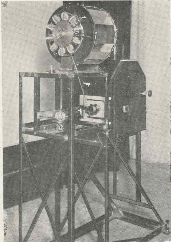
Scophony 5ft. x 4ft. Screen Television Projector for 405 line interlaced scanning.
