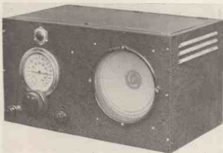
Only three controls are required, these being screen voltage, tuning and cathode bias. The cabinet is a special Eddy-stone product which is supplied complete with dial and loudspeaker fret.
