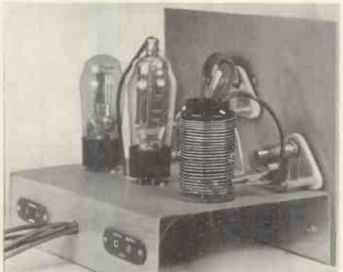
Most of the connections are beneath the baseplate, so giving the finished receiver a commercial appearance.
