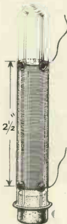
The Chatterton's compound for fixing the wire can easily be seen. As a general rule 30 gauge wire will occupy 2\frac{1}{2} inches of former.
