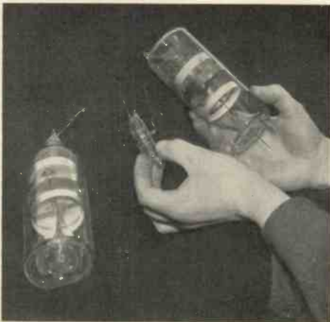
The Farnsworth electron-multiplier. A full description of this new tube is given on page 195.
