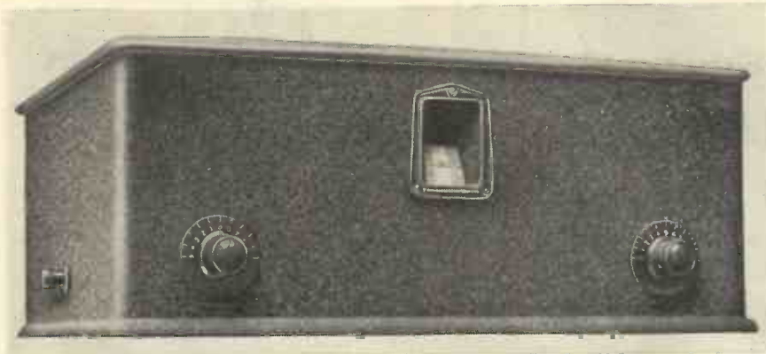
The Eddystone receiver has been designed for tropical use; it is particularly selective on the broadcast bands.
