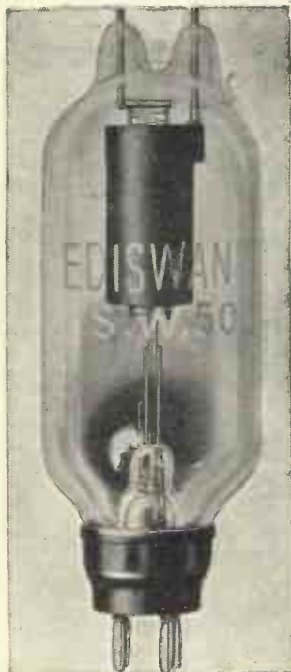
One of the very latest short-wave valves. This S.W. 50 has a graphite anode and a thoriated tungsten filament. Dissipation up to 40 watts at ten metres is possible.
