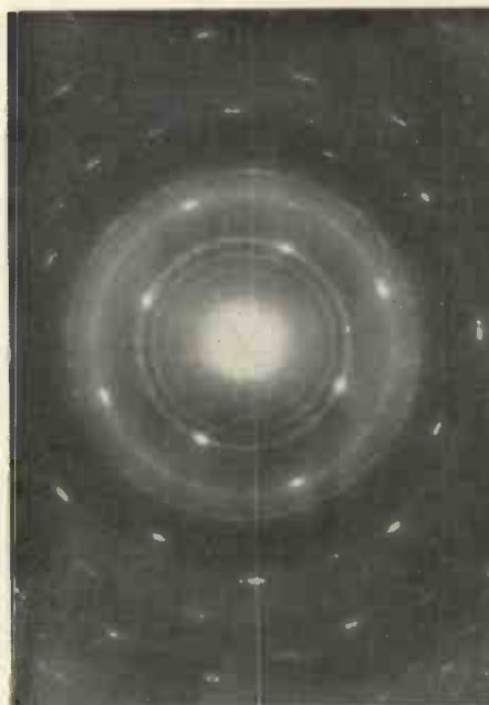
Fig. 3.—Electron-pattern from film containing an aluminium crystal (spot pattern) and scattered aluminium and aluminium-oxide (ring pattern) (Photograph by courtesy of Professor G. I. Finch of the Royal College of Science).
