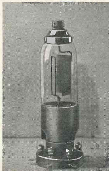
A small type of caesium photo-electric cell. This has a plate cathode and is suitable for televising films.
