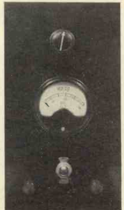
Fig. 1.—Photograph showing the recommended method of mounting ordinary measuring instruments.
